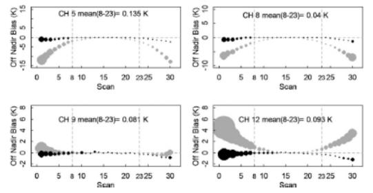
• (Advanced Microwave Sounding Unit) AMSU-A onboard six POES satellites were inter-calibrated using the Integrated Microwave Inter-Calibration Approach (IMICA)
