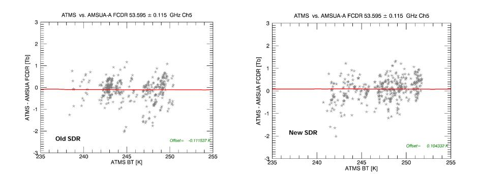
Comparisons show inter-comparision with FCDR is capale of revealing changes in SDR processing. In this case shows change in bias from old version SDR to new version SDR
