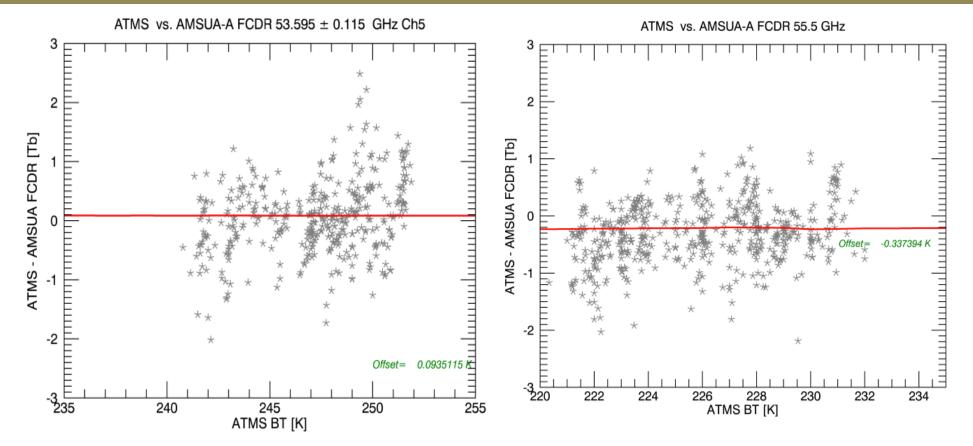
Shows the temperature dependence of bias of ATMS. Close to pre-launch levels (Weng et al, 2016) ATMS-SDR and FCDR both very close to maintain pre-launch behavior in space.
